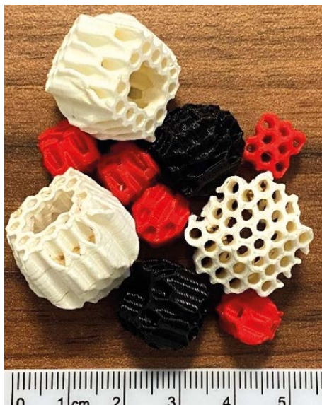
Figure 2: 3D printed lost circulation shapes
